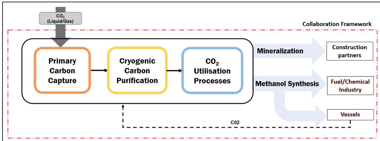
In the first stage of the CCUS system – Primary Carbon Capture. Membrane separation technology is currently limited by the selectivity of currently available membrane materials as well as the high cost of materials. One of the most promising gas separation method is using polymeric membrane that acts as the filter for the separation CO<sub>2</sub>/N<sub>2</sub> mixtures and generates a specific gas rich permeate.
